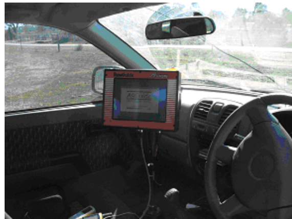
Photos: Left – GPS base station setup; Top Right – GPS antennae and UHF radio antennae, the radio is the communication link between the stationary base station and the mobile rover unit; Bottom Right – the rover unit computer & control interface.
