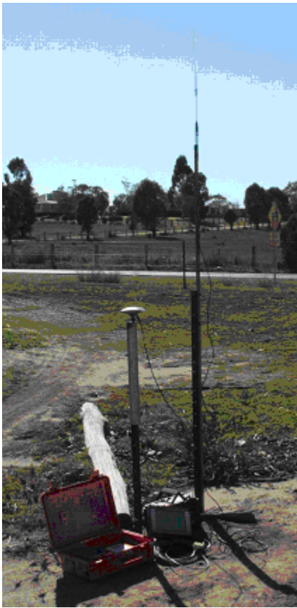
Photos: Left – GPS base station setup; Top Right – GPS antennae and UHF radio antennae, the radio is the communication link between the stationary base station and the mobile rover unit; Bottom Right – the rover unit computer & control interface.
